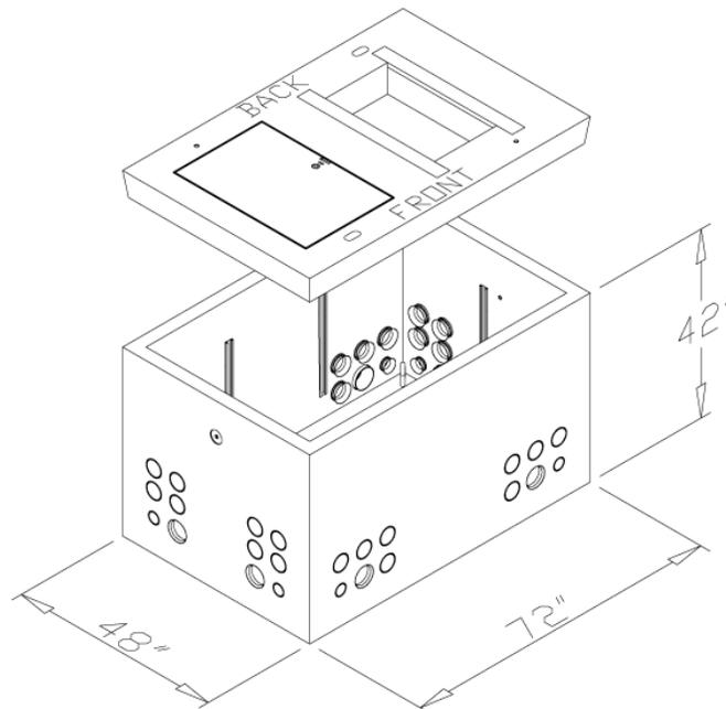
**Figure 54—A Typical Vault for a Single-Phase Sectionalizing Cabinet (SI# 7992975)**
