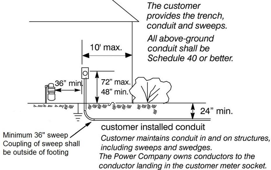
Figure 32—Wall-Mounted Meter Socket Location for Underground Service
