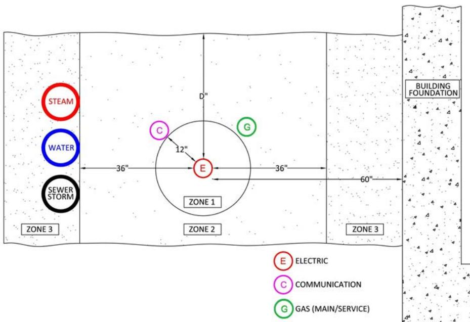
**Figure 9—Minimum Separation of Paralleling Lines and Structures**
