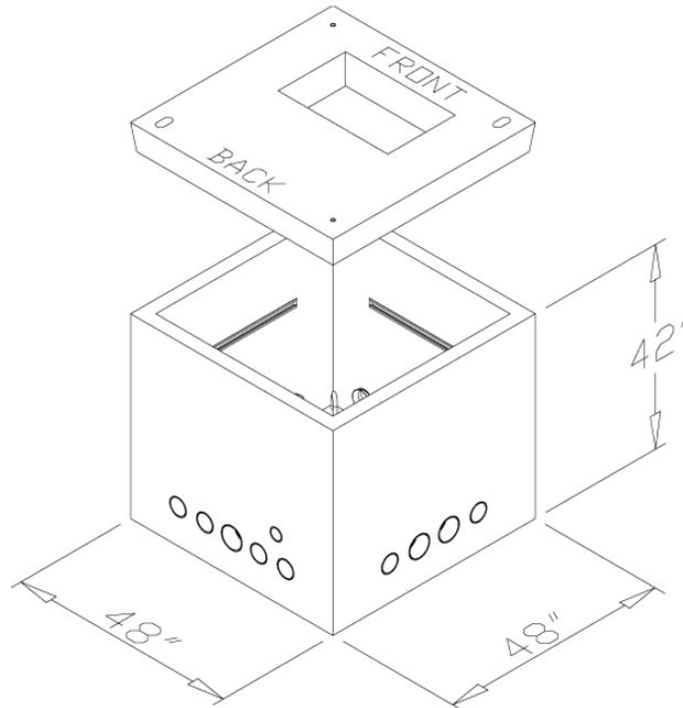
**Figure 50—A Typical Vault for a Single-Phase Pad-Mounted Transformer
