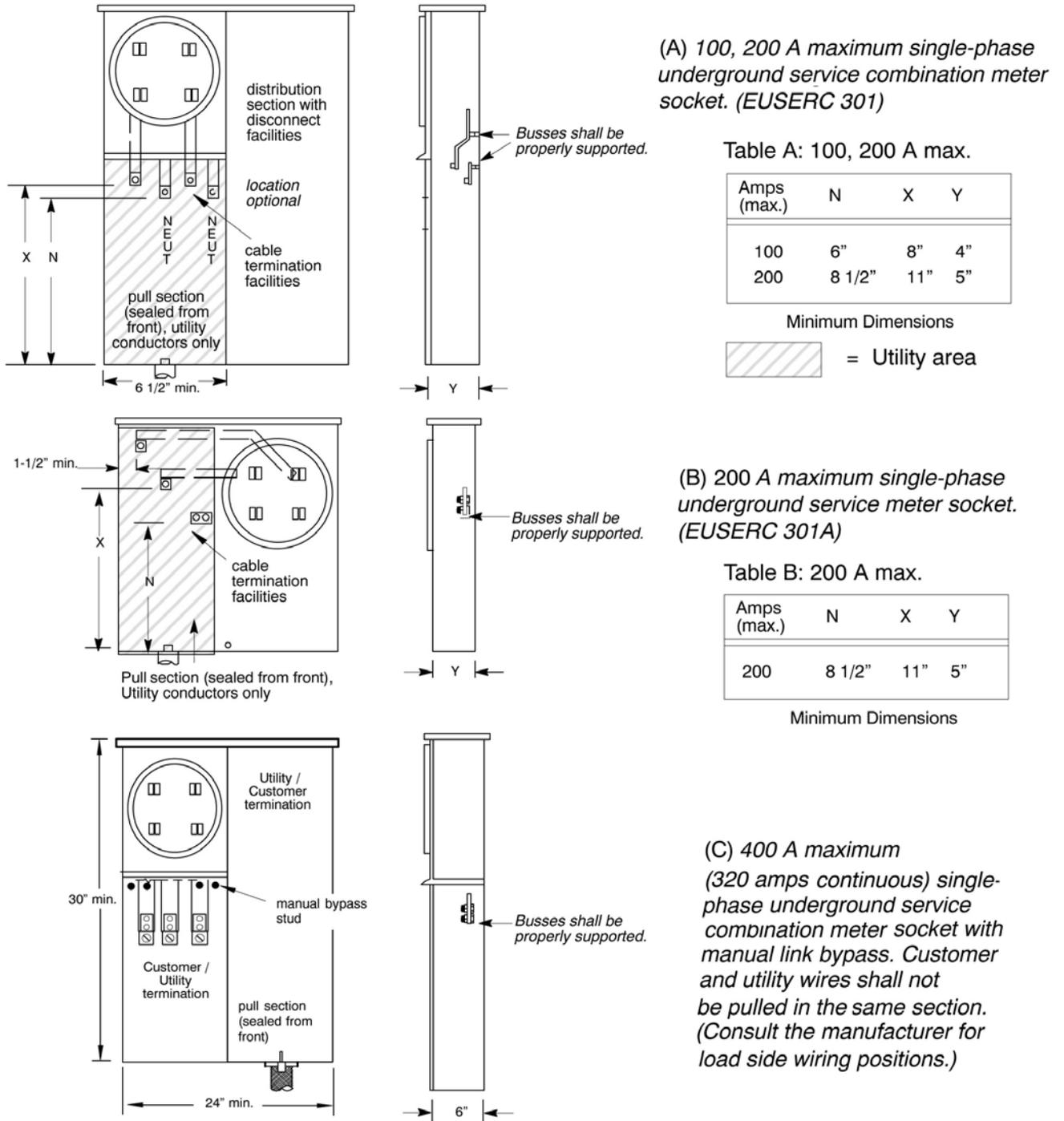
**Figure 34—Residential Underground Approved Meter Sockets**
