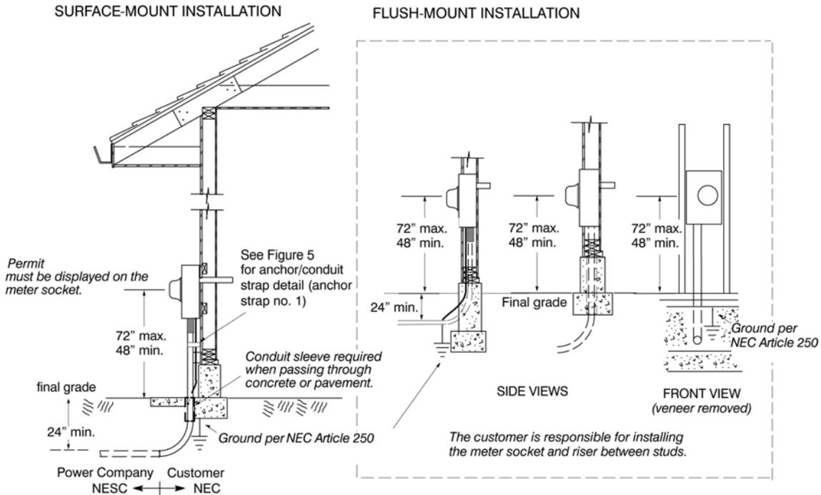
**Figure 33—Underground Service to Wall-Mounted Meters**
