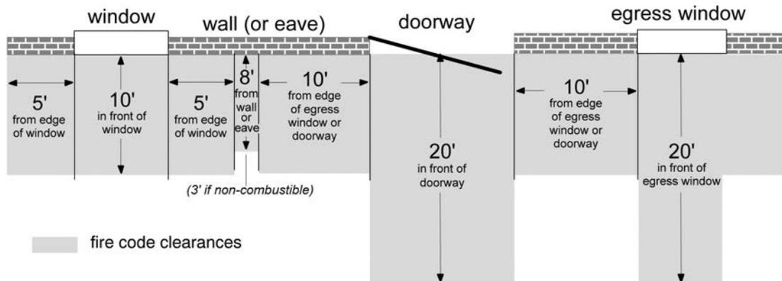
**Figure 42—Clearances Between Equipment and Structures**
