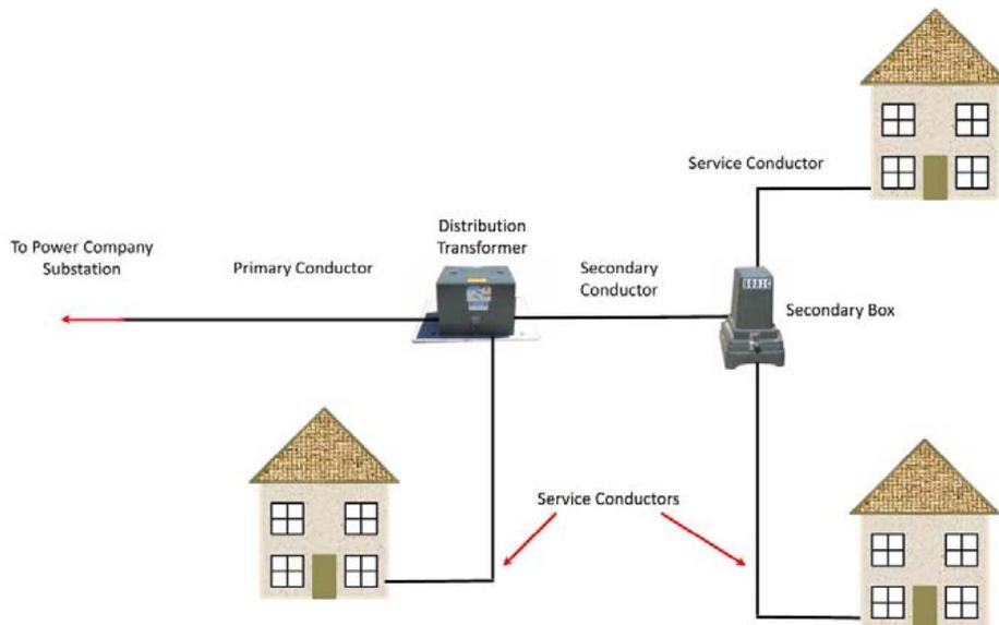
**Figure I—Primary, Secondary, and Service Conductor Schematic**
