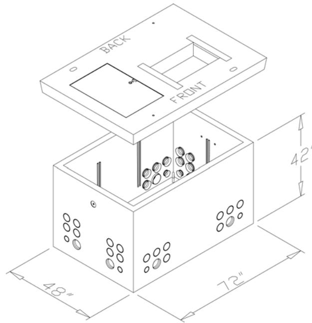
**Figure 51—A Typical Vault for a Single-Phase, Pad-Mounted Transformer with Opening (SI# 7992977)**
