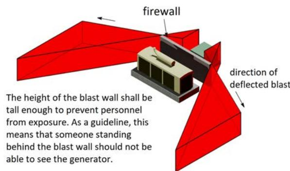
**Figure 43—Typical Firewall**
