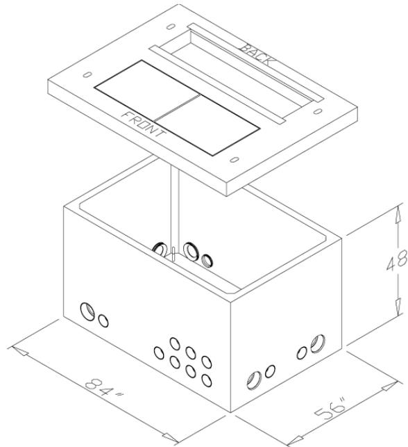
**Figure 53—A Typical Vault for a 15 kV Three-Phase Sectionalizing Cabinet (SI# 7992605)**
