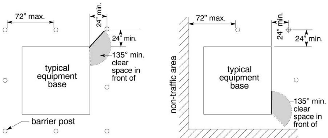
**Figure 44—Barrier Post Layout and Clearances**
