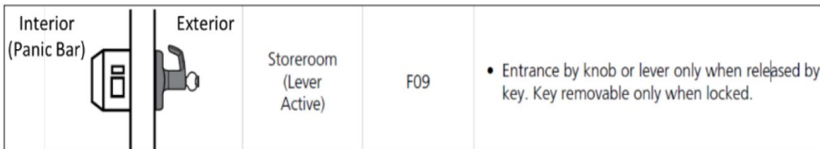
Figure 1 – Equipment Room Door Lockset Functionality
