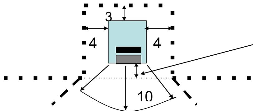
**Figure 1 – Clearances Around Nonmetallic Equipment in an Enclosed Space**
