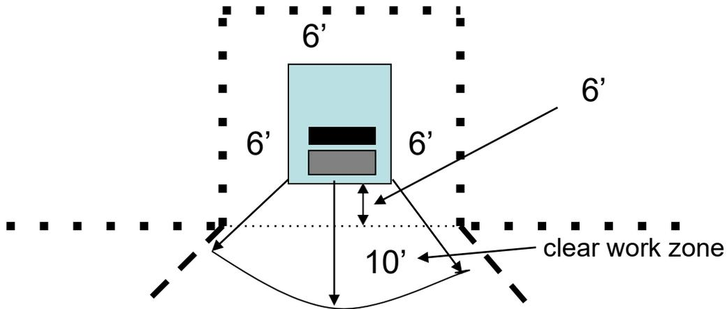
**Figure 2 – Clearance Around a Metallic Fenced Enclosure**
