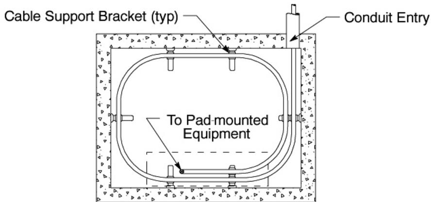
**Figure 8—Equipment Base Cable Training and Support**
