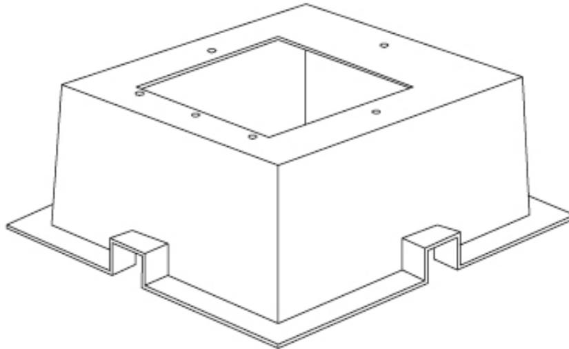
**Figure 2—Typical Equipment Box Pad**
