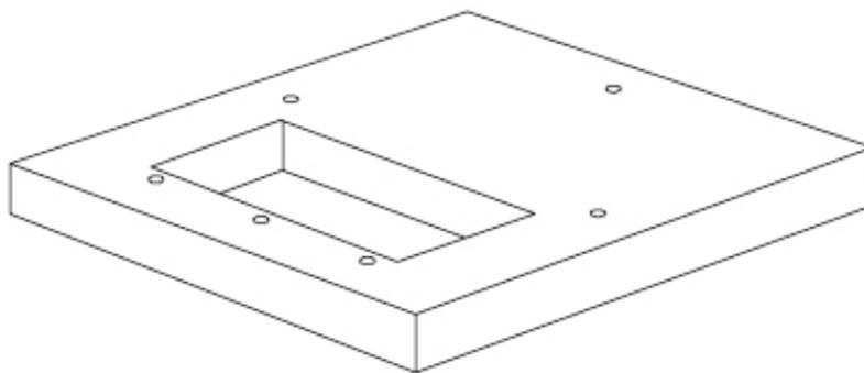
**Figure 1—Typical Equipment Flat Pad**
