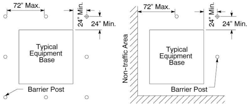
**Figure 11—Typical Barrier Post Layouts**
