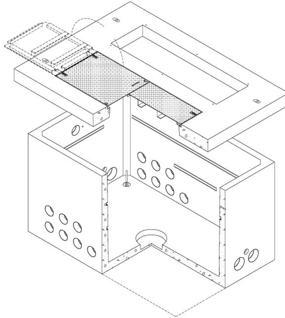
**Figure 3—Typical Equipment Padvault**
