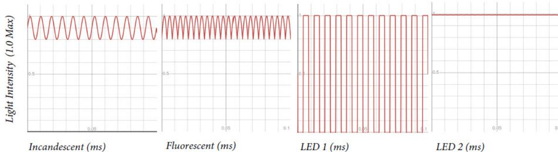
**Figure 1—Light Output Variability of Incandescent, Fluorescent, and LED types (1 and 2), Left to Right**
