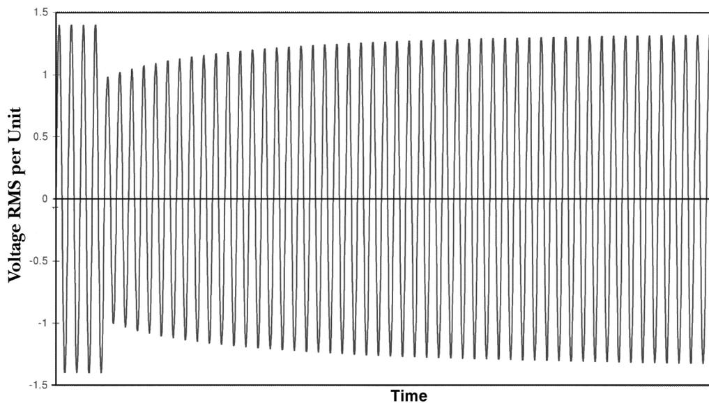
**Figure 2—Typical Motor Start Voltage Waveform**
