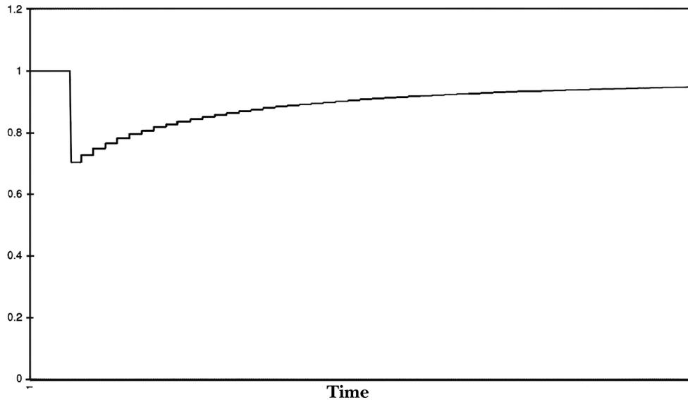
**Figure 1—Typical Motor Start Voltage Profile**
