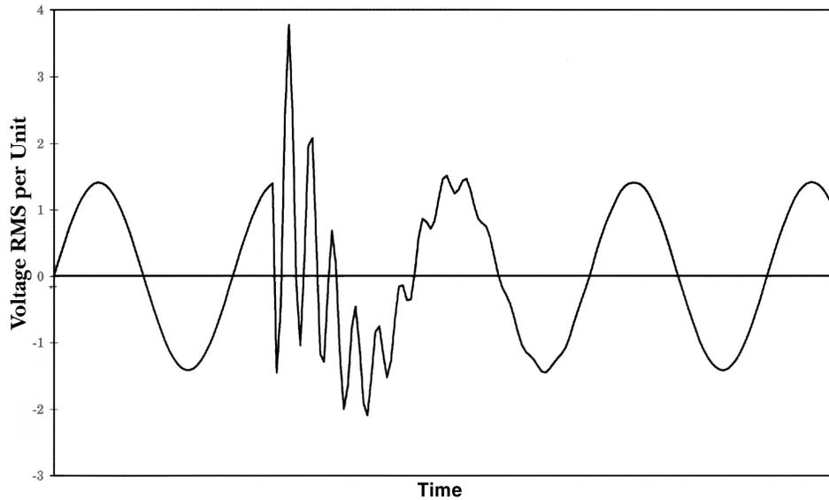
**Figure 3—Typical Capacitor Bank Closing Voltage Waveform**
